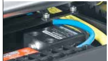
Two inner magnetic switches factory-set at the feeder's stroke limits prevent overtravel. Two outer fail-safe limit switches automatically engage the brake.
