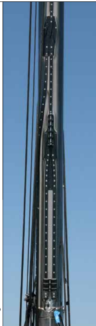
The Trysail Switch system integrates with the Switch T-Track Battcar system by sharing a single track to reduce weight aloft.
