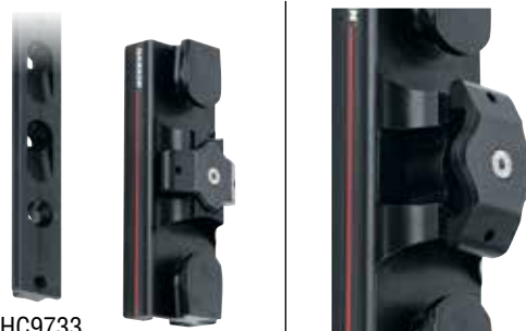
To lock pin in up position, pull the handle up with a lanyard or by hand and twist 90 degrees.
