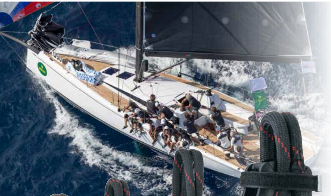
A fixed Velcro strap keeps sideplates aligned and securely closed under high loads.
