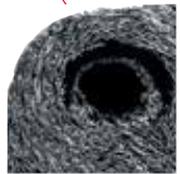
Carbo composite: Sideplates, sheave
