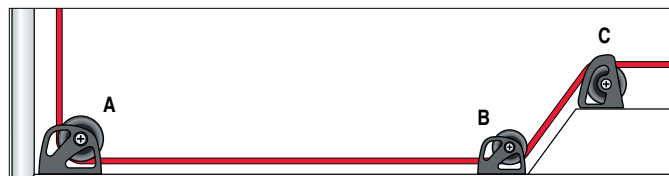
Over-the-Top: Special "over-the-top" blocks are required to route lines over an outside corner like the front of a doghouse or coaming.
