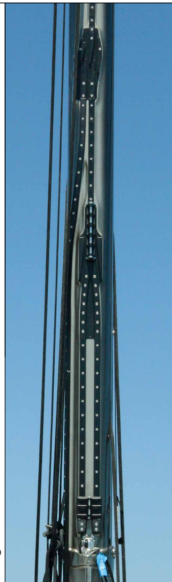
The Trysail Switch system integrates with the Switch T-Track Battcar system by sharing a single mast track to reduce weight aloft.
