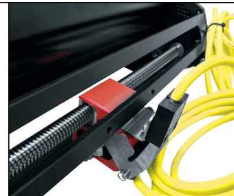
The screw design positions the screw close to the drum, reducing winch size.
