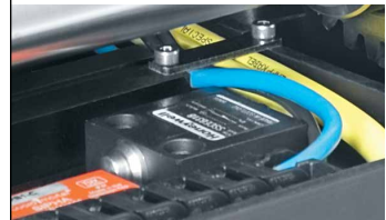
Two inner magnetic switches factory-set at the feeder's stroke limits prevent overtravel. Two outer fail-safe limit switches automatically engage the brake.
