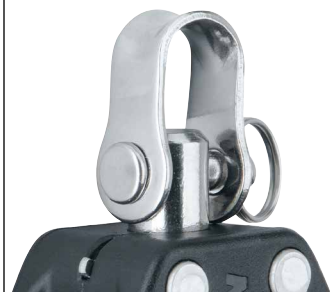
Switch locks shackle in front or side positions, or lets block swivel to keep line from twisting.
