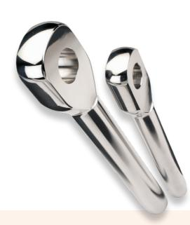
Our stainless steel swage terminals have been designed for use with 1×19, 7×19, 7×7 and compacted strand stainless steel wire rope and can be installed using both rotary & fixed die swaging machines.
